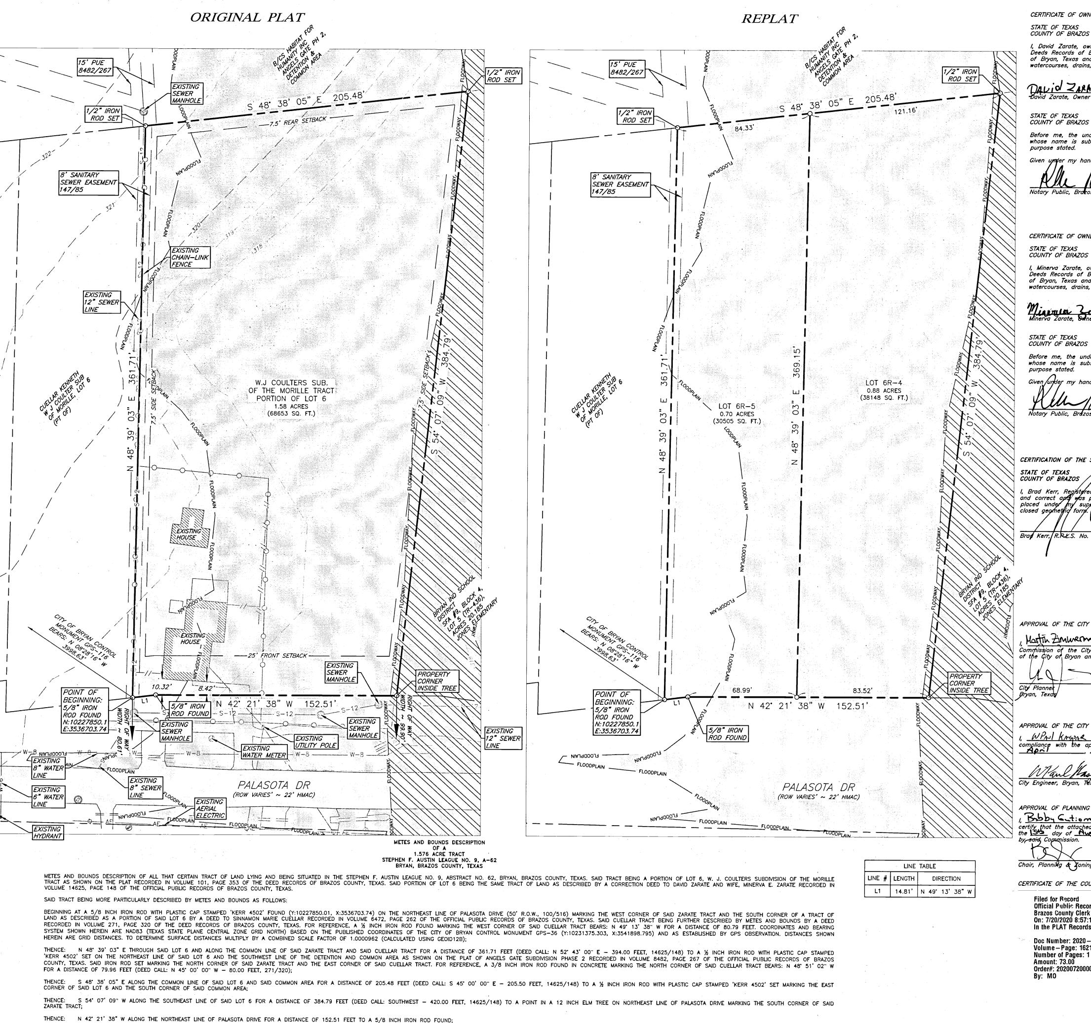
THENCE: N 49° 13' 38" W CONTINUING ALONG THE NORTHEAST LINE OF PALASOTA DRIVE FOR A DISTANCE OF 14.81 FEET TO THE POINT OF BEGINNING CONTAINING 1.576 ACRES OF LAND, MORE OR LESS, AS SURVEYED ON THE GROUND JULY 2018.
